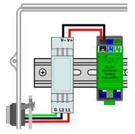
4. If connecting multiple transmitters, use parallel connections between all PWR terminals.
