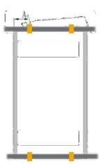
Test load: positive 1600Pa negative 1000Pa Safety factor: 1.5
