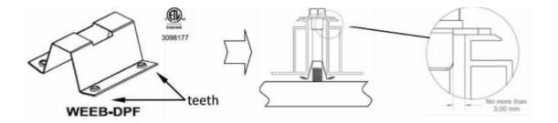
Use WEEB-DPF to bond solar modules to module mounting brackets (grounding part is tested to UL467)
