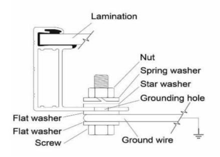
2) Use WEEB-DPF to bond solar modules to module mounting brackets (grounding part is tested to UL467)
