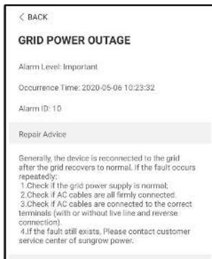
figure 7-8 Detailed Fault Alarm Information
